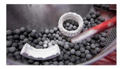
14.7. Stratasys post-processing of 3D printed models on Polyjet technology
