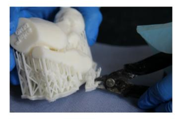
Carefully remove supports from delicate areas, use light pressure when snipping. Cut from the bottom of the support moving closer to the surface to avoid breaking off small features.
