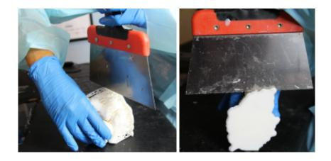
Use the wire snips to slowly release the supports from the model, breaking off small sections until complete.
