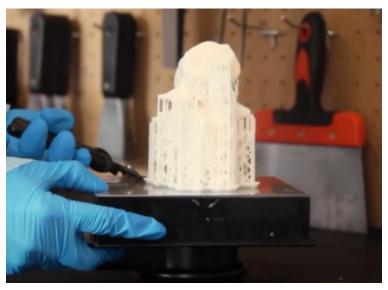
Carefully do this over a table to avoid the model dropping from a height. Using a round edged scraper to scrape off any excess left behind on the build plate. Scrape away from yourself.
