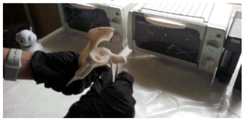
When all supports have been successfully removed, wipe over the model with a microfibre cloth and IPA to remove any excess tackiness.
