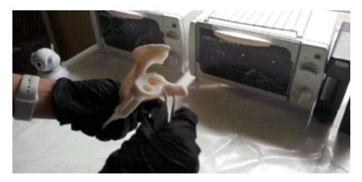
When all supports have been successfully removed, wipe over the model with a microfiber cloth and IPA to remove any excess tackiness.
