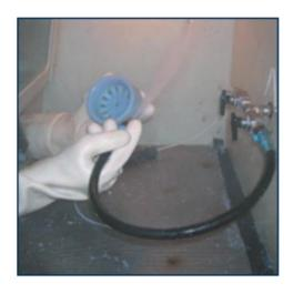
Immerse the model in the sodium hydroxide solution for up to two hours, depending on the model size and type.
